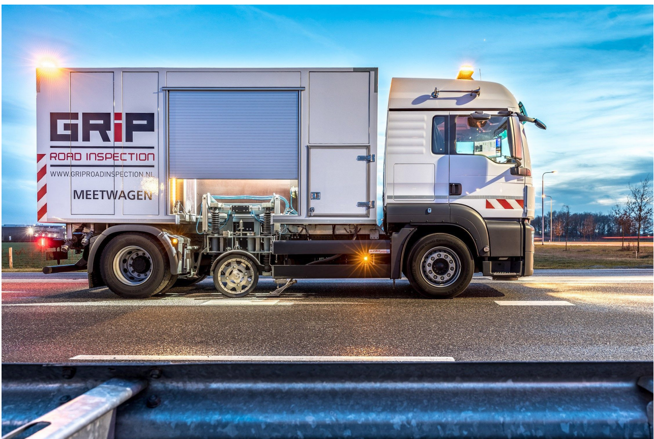
Figure 5: Sideway Force measure truck
