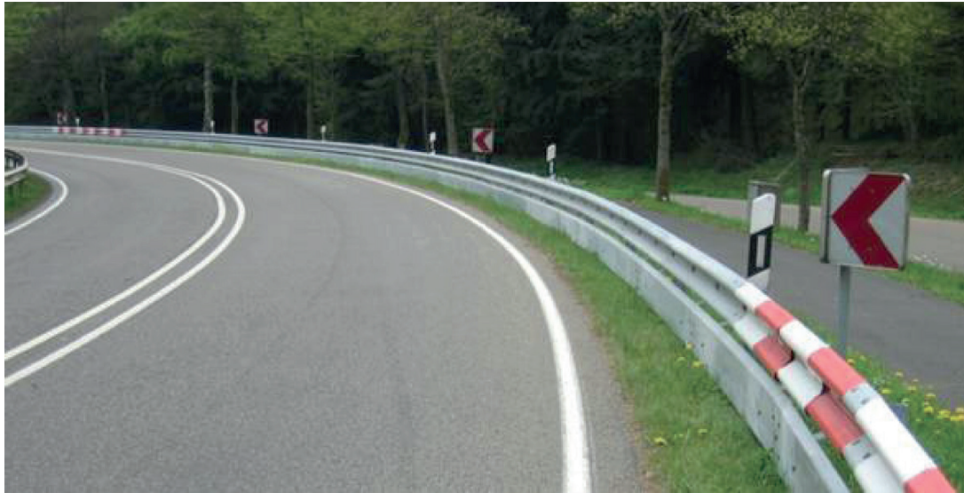
Figure 2 : Steel guardrail with MPS system
