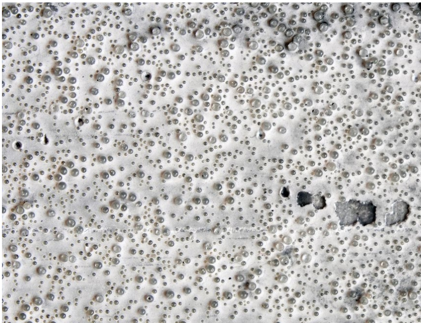
Figure 2. Test panel after 12 million tyre rollovers. Drop-on glass beads protect the underlying paint from abrasion.
